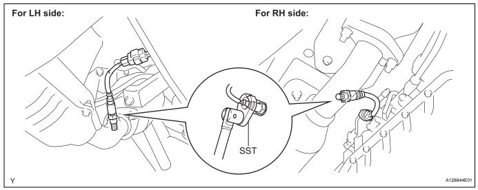
(b) Connect the 2 heated oxygen sensor connectors.
